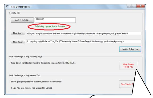
**4.** Click on "Write Protect T-Safe Key" after preparing the dongle to ensure that end user cannot use it for any other purpose.
