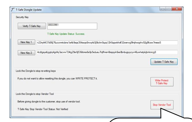
5. Click on "Stop Vendor Tool" after you encrypt all your desired files and before giving dongle to the customer to prevent the customer from accessing the Vendor Tool.
